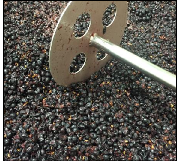
Hand punchdowns are done 1-3 times per day, depending upon the stage of fermentation
